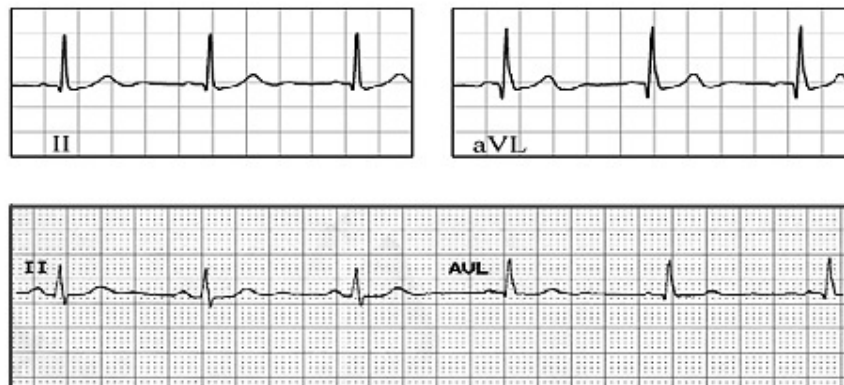
Fig. 7 Comparison of two vectors from a pair of EPIC sensors (top) and two conventional Ag/AgCl electrodes (bottom)
